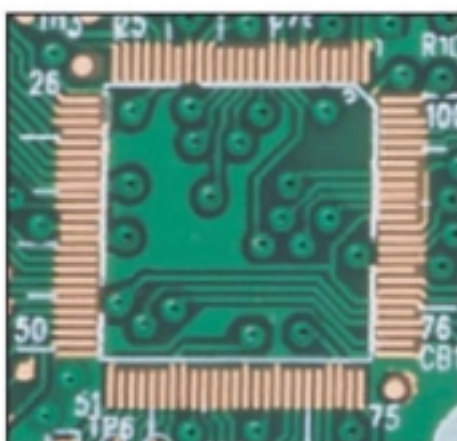
Close-up detail of power-supply PCB (below) showing 16 mil (0.4mm) pitch pads and STH's.
