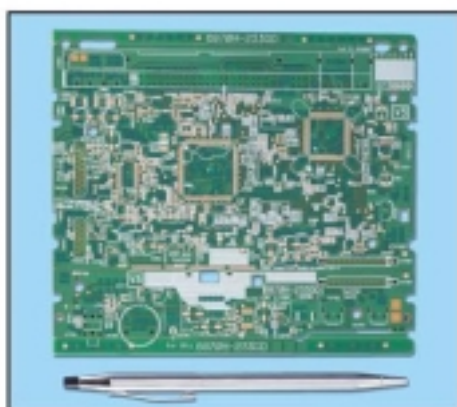
Complex Double-sided PCB for DVD with over 850 Silver-Through-Hole connections.
